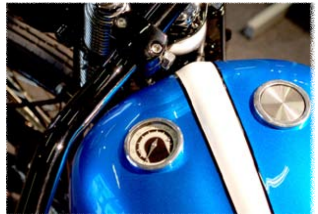
Speedometer »mst Speedster«, by Motogadget GmbH, 24 mm deep, Ø 49 mm, Germany
